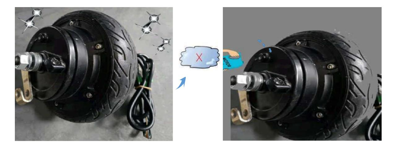
2.Must keep the motor wheeldry. Away from water. 3.Add lubrication oil on motor wheel every 1-2 months.
