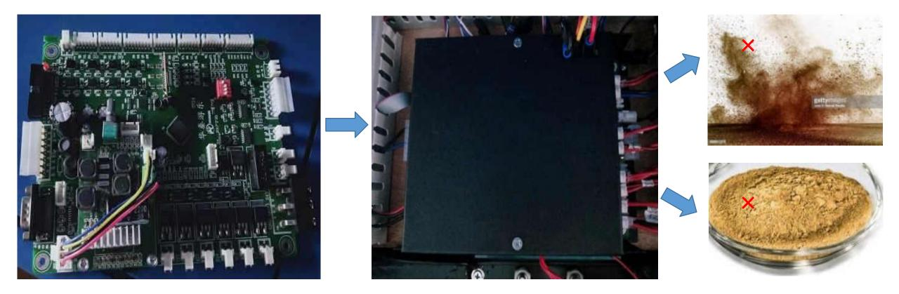
12. The mainboard box must be covered after maintenance is completed.
