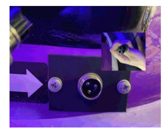
6.Must connect AC(charging plug) first, then connect DC(plug the machine), instead, It will cause damage to the machine.
